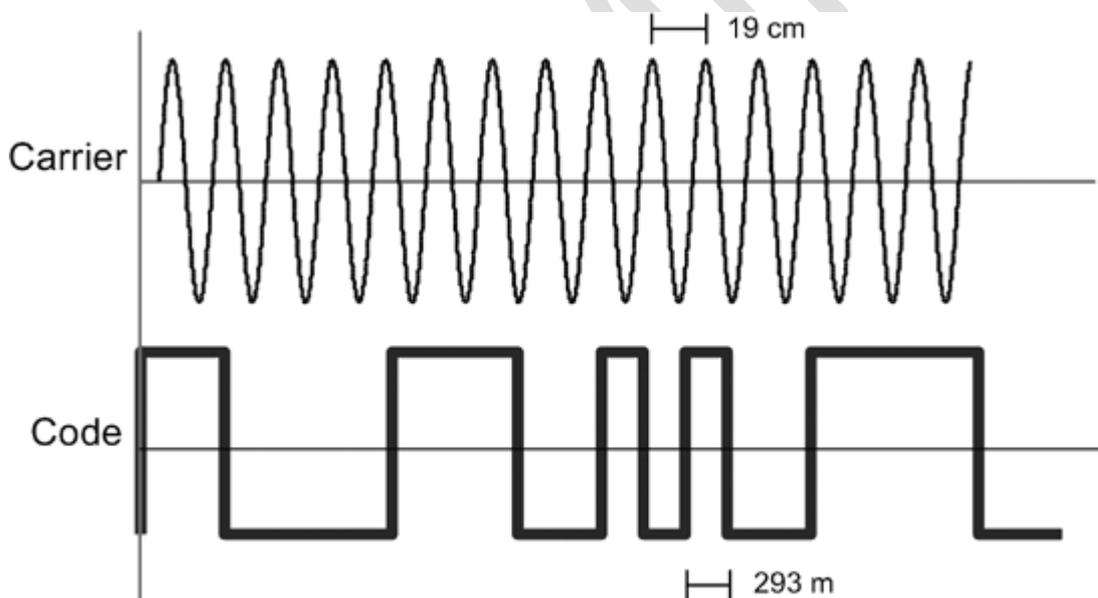
But the carrier phase measurement contains uncertainty which is the number of cycles between the satellite and the receiver. It is called ambiguity.
