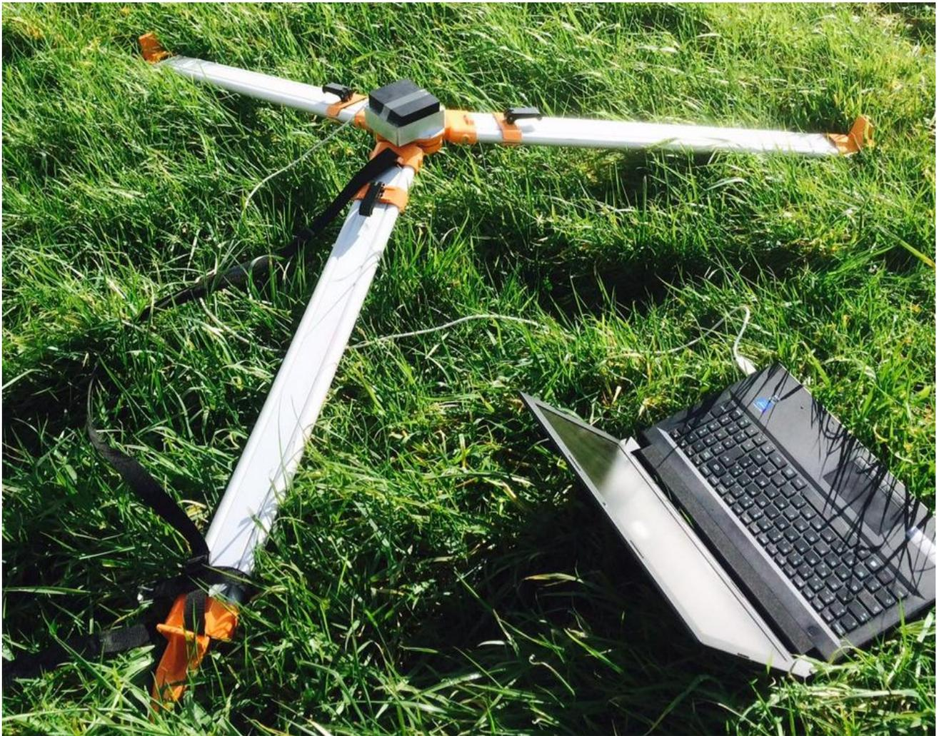
Between 2 geocubes placed at 1m height the range is approx 150m,
